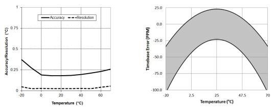
Plot A: Internal Temperature Accuracy & Resolution
